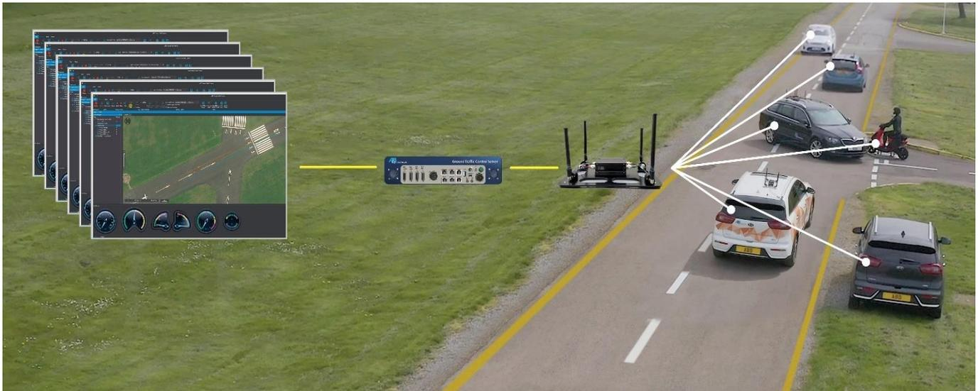
The Ground Traffic Control (GTC) System is the next generation software and hardware solution for monitoring, commanding and coordinating proving ground vehicle testing. GTC is a comprehensive package for all vehicle traffic at a proving ground including: robot-controlled vehicles, ADAS platforms, human driven vehicles and fixed proving ground infrastructure.
